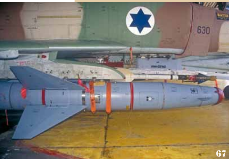
66: TV guided RAFAEL AGM-142A Popeye attached to special purpose inner wing pylon with movable suspensions;
