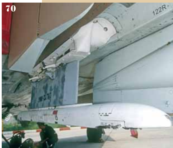
70+71+72: The Israeli designed Sparrow bay missile adaptor with standard LAU-7/A launch rail and AIM-9D 'Decker' AAM. The missile adaptor is attached to the standard suspension used with the ECM pods and can only carry the AIM-9 AAM.
