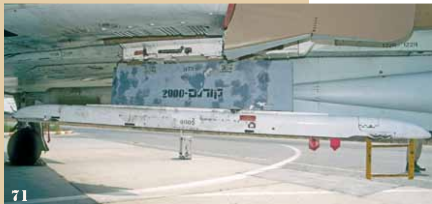
66: TV guided RAFAEL AGM-142A Popeye attached to special purpose inner wing pylon with movable suspensions;
